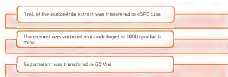
Fig. 2b: Clean-up procedure after surface sediments extraction. Source: Guided and informed by Anastassiades et al., (2003)
