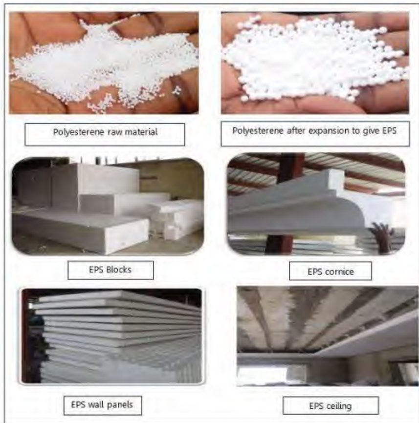
Fig. 2: EPS elements used at Citec Mborra Mount Pleasant Estate Abuja. Source: Researcher's Archive, 2023.
