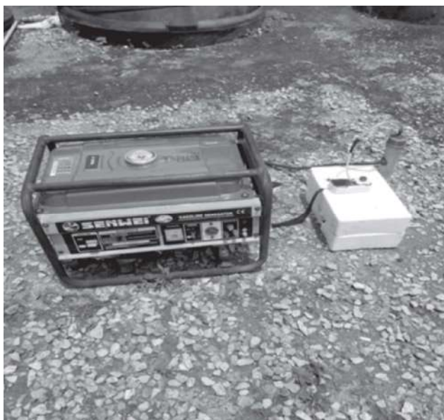
Plate 1: Experimental Setup for the Investigation of the activated carbon removal efficiency of the toxic gaseous emissions from gasoline-powered generator
